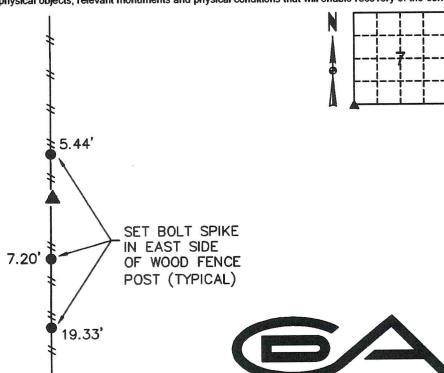
**SW CORNER** SECTION 7-T74N-R18W SET 3/4" REBAR **W/PURPLE CAP #19968**
