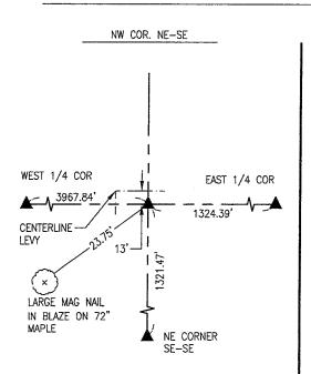
DECEMBER 15, 2023 SET 5/8" X 30" REBAR PLS #19960 AT THE MIDPOINT OF A LINE CONNECTING THE EAST 1/4 CORNER AND CALCULATED POSITION FOR THE CENTER OF SECTION
