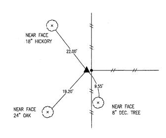
OCTOBER 2022 COUNTY ENGINEER DOES NOT HAVE RECORDS OF THIS CORNER BEING SET. SET 5/8" REBAR WITH YELLOW CAP #19960 AT ANCIENT 3-WAY FENCE CORNER. THE DISTANCE SOUTH TO FENCE CORNER AT THE SE CORNER OF THE NORTH 6 ACRES OF THE SW-NE OF SEC. 7-75-18 MEASURES WITHIN A FOOT OF RECORD DISTANCE.
