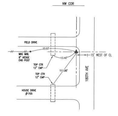
FEBRUARY 2022 FOUND 5/8" REBAR LEANING FROM COUNTY ENGINEER TIES. REMOVED REBAR AND DUG DOWN TO WPA CONCRETE MONUMENT 1.5' DEEP. RESET 5/8" REBAR ABOVE MONUMENT AND TIED OUT CORNER.
