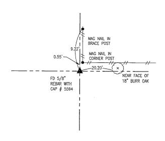
FOUND 5/8" REBAR WITH YELLOW CAP #5594 AT TWO—WAY FENCE CORNER. CORNER HAS BEEN USED FOR SURVEYS RECORDED IN BOOK 2004 PAGE 5389 AND BOOK 2004 PAGE 5245. ACCEPTED CORNER AND TIED OUT. THIS CERTIFICATE IS BEING PREPARED BECAUSE THERE IS NO CERTIFICATE FOR THE CORNER ON FILE WITH THE MARION COUNTY RECORDER.
