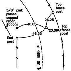
NOTE: ALL TIES ARE PLUMB MEASUREMENTS TO ORANGE SURVEY MARKER UNLESS NOTED.
