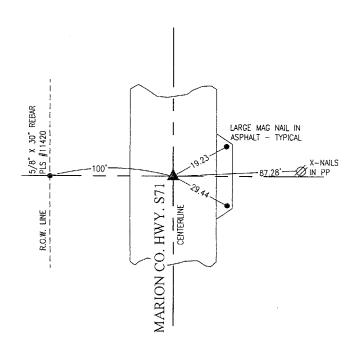
AUG. 23, 2021 CORNER WAS LOST BY RESURFACING PROJECT. RESET AT MIDPOINT OF EAST LINE OF NE 1/4.
