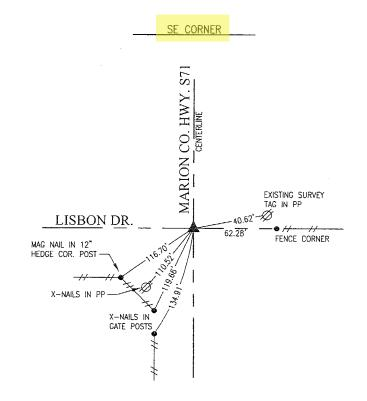
AUG. 23, 2021 SET LARGE MAG NAIL IN CL OF PAVING AND FENCELINE TO EAST.
