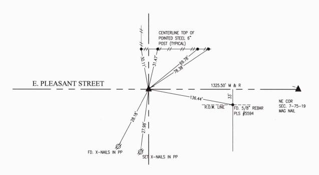
JULY 12, 2022 RESET MISSING CORNER RECORD DISTANCE FROM NE CORNER SECTION 7 AND 33.00' NORTH OF FOUND PROPERTY CORNER.
