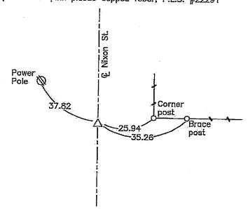
NOTE: ALL TIES ARE PLUMB MEASUREMENTS TO ORANGE SURVEY MARKER UNLESS NOTED.
