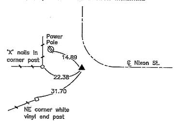
NOTE: ALL TIES ARE PLUMB MEASUREMENTS TO ORANGE SURVEY MARKER UNLESS NOTED.
