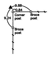
NOTE: ALL TIES ARE PLUMB MEASUREMENTS TO ORANGE SURVEY MARKER UNLESS NOTED.
