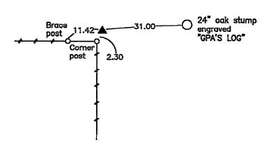
NOTE: ALL TIES ARE PLUMB MEASUREMENTS TO ORANGE SURVEY MARKER UNLESS NOTED.
