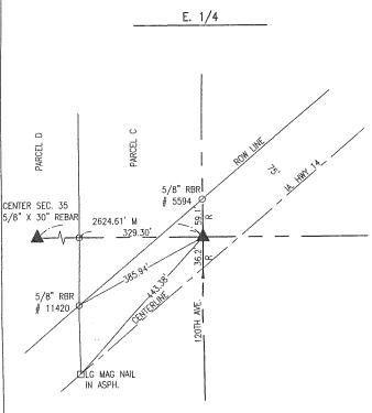
FOUND 5/8" X 12" REBAR W/ CAP# 5594 ABOVE CONC. MONU. WE SET A 5/8" X 15" REBAR 0.3' DEEP ABOVE THE EXISTING REBAR. WE PROBED DOWN BELOW EXISTING REBAR AND HIT C.M.
