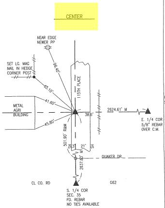
AT CENTER SECTION 35 WE FOUND THE 1/2" REBAR INSIDE A 1-1/2" PIPE (ONLY 10" +- LONG) REABAR BENT AND PIPE LEANING SOUTH STRAIGHTEN TO FIT TIES THEN DECIDED TO REPLACE WITH A NEW 5/8" X 30" REBAR W/ CAP # 11420 0.5' DEEP.
