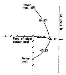
NOTE: ALL TIES ARE PLUMB MEASUREMENTS TO ORANGE SURVEY MARKER UNLESS NOTED.
