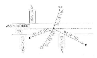
NOTE: ALL DISTANCES MEASURED HORIZONTAL UNLESS OTHERWISE NOTED. S&A\_Section Certificate\TWP\_RNG\_SEC\_PROJECT\_NUM\76\_21\_15\_NWCorNESW\_1170319.dgn
