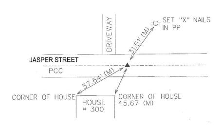
NOTE: ALL DISTANCES MEASURED HORIZONTAL UNLESS OTHERWISE NOTED. SEC\_PROJECT\_NUM\76,\_21\_15\_.W\_1170319.dgn
