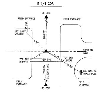
OCT. 23, 1940-MARION COUNTY ROAD DEPT: FOUND FIELD BOULDER ON NORTH SIDE OF WATKINS TILE 1-2 1/2" & 1-2" ALSO BROKEN COAL ROCK. SET C.M. 8" DEEP OVER 1-2 1/2" TILE IN PLACE AND SET FIELD BOULDER ON TOP OF C.M.
