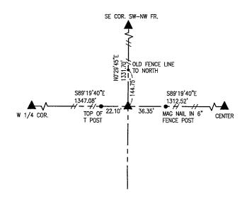
JAN. 26, 2022—PLS 14416: SET 5/8" X 30" REBAR WITH YPC #14416 AT INTERSECTION OF LONG STANDING FENCE LINE NORTH WITH LINE BETWEEN CENTER AND W 1/4 CORNER.
