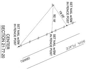
SET 1/2" x 30" REBAR W/YELLOW PLASTIC CAP #15270. SET SW CORNER OF THE SE1/4 OF THE NW1/4 BY PROJECTING THE CENTERLINE OF 90th PLACE TO THE MIDPOINT OF THE SOUTH LINE OF THE NORTHWEST 1/4, THE SOUTH LINE BEING PARALLEL TO THE NORTH LINE OF THE NORTHWEST 1/4, THEN DOUBLING THE DISTANCE TO THE CENTER OF THE SECTION.
