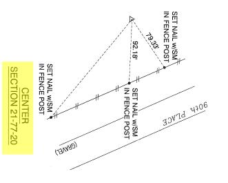
SET 1/2" x 30" REBAR W/YELLOW PLASTIC CAP #15270. SET SW CORNER OF THE SE1/4 OF THE NW1/4 BY PROJECTING THE CENTERLINE OF 30th PLACE TO THE MIDPOINT OF THE SOUTH LINE OF THE NORTHWEST 1/4, THE SOUTH LINE BEING PARALLEL TO THE NORTH LINE OF THE NORTHWEST 1/4, THEN DOUBLING THE DISTANCE TO THE CENTER OF THE SECTION.
