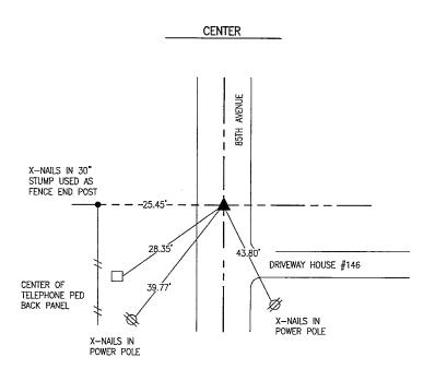
MARCH 2021 FD 2" PIPE 12" DEEP IN CENTERLINE OF ROAD IN LINE WITH FENCE TO THE WEST. THE DISTANCE SOUTH TO THE SOUTH 1/4 (5/8" REBAR OVER C.M.) 2636.79' FITS WITHIN REASON. ACCEPTED MONUMENT AND TIED OUT.
