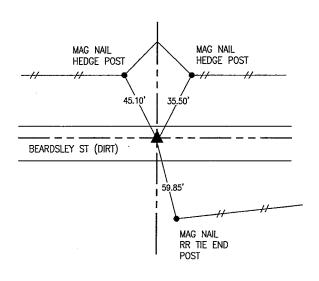
FOUND BENT WAGON HUB WITH WPA CONCRETE MONUMENT 6" SOUTH FROM COUNTY ENGINEER TIES. TOP OF C.M. IS 12" DEEP. THE WAGON HUB IS THE CORNER AND MADE NOTCH AT LOCATION USED. MONUMENT IS APPROXIMATELY 5' NORTH OF ROAD CENTERILINE.
