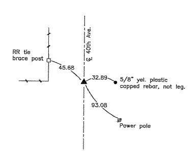
NOTE: ALL TIES ARE PLUMB MEASUREMENTS TO ORANGE SURVEY MARKER UNLESS NOTED.
