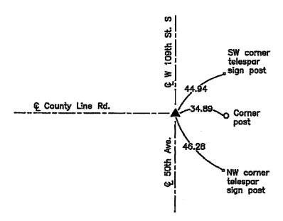
NOTE: ALL TIES ARE PLUMB MEASUREMENTS TO ORANGE SURVEY MARKER UNLESS NOTED.
